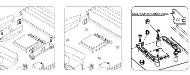
REMOVE AMD AM4 plastic brackets, KEEP the back plate, install AM4 metal brackets with AM4 screws and AM4 plastic standoffs
