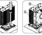
Apply thermal grease on CPU, install the heatsink with a screw driver, and install fans on heatsink with fan clips
