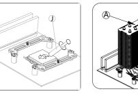
Apply thermal paste on CPU, install the heatsink with a screw driver, and install fans on heatsink with fan clips
