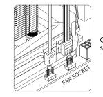
Connect 4-Pin PWM fan header to motherboard CPU\_FAN socket to power and control fan speed.
