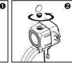
Tear off the warranty sticker and loosen the refill cap carefully with a coin or screwdriver.
