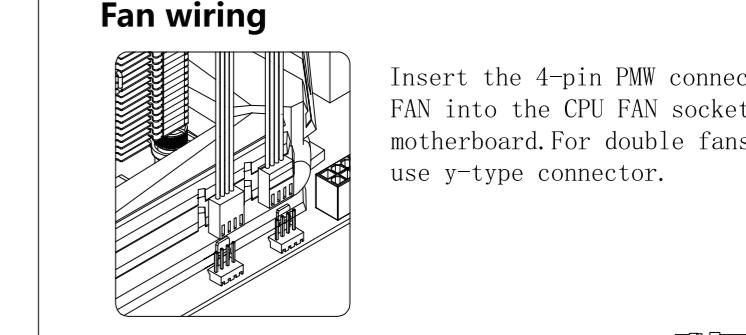
Insert the 4-pin PMW connector of the FAN into the CPU FAN socket of the motherboard. For double fans, please use y-type connector.
