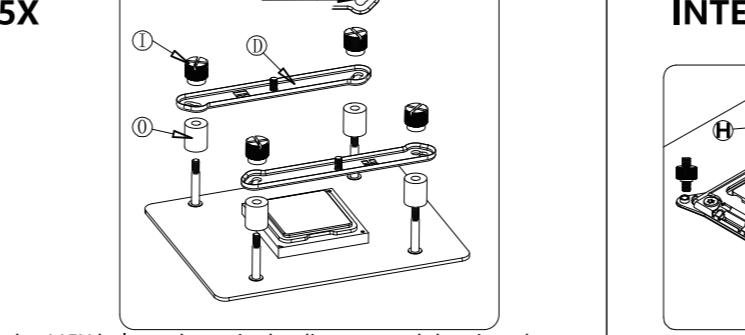
Install the backplane into the 115X hole as shown in the diagram, and then jam the backplane with the O-shaped plastic pad. Then place the backplane on the back of the motherboard, place the 115X rubber column to tighten the stud, and then fix the support with nuts (the support hole is aligned with 115X).
