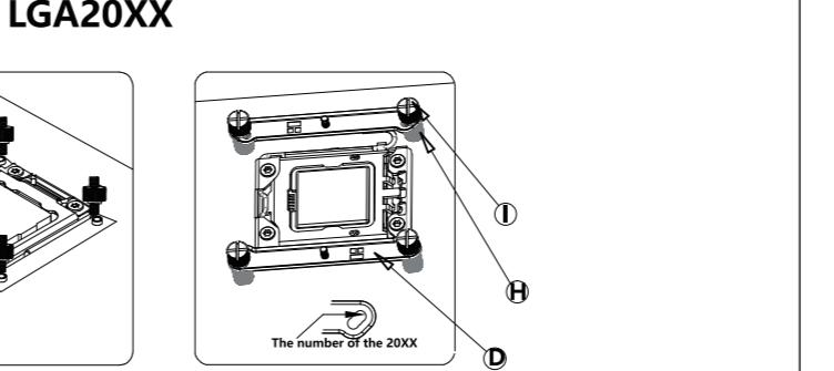
Thread in the LGA20XX screws; put on the brackets and then tightening with nuts.
