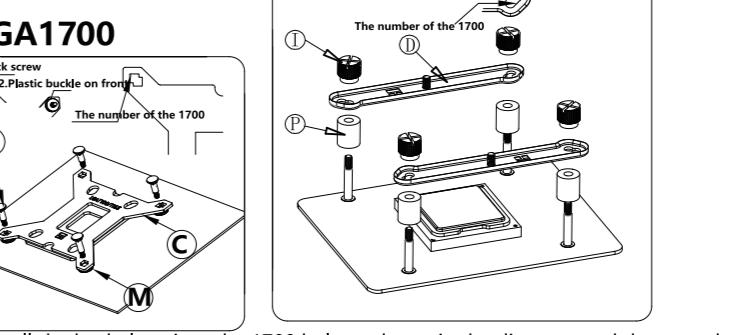
Install the backplane into the 1700 hole as shown in the diagram, and then use the O-shaped plastic pad to jam the backplane. Then place the backplane on the back of the motherboard, place the 1700 plastic column, and fix the support with screws (the support hole is aligned with 1700).
