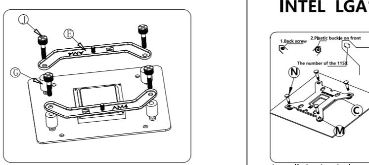
Remove plastic retention bracket, but keep the backplate; secure the brackets using the AM4 screws.
