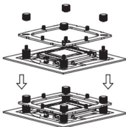
Step 5 : Place the Anchoring Bracket Mount on top of the four Screw Pillars. Tighten the 4 Screw Pillars with the Thumbscrew Caps.
